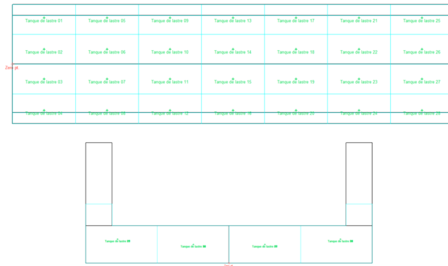
Figure 2. Ballast-tank arrangement (MAXSURF): plan view of the 28 ballast tanks (top) and transverse section (bottom). Source: The authors.
